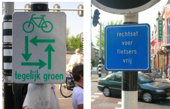
Green light for cyclists in all directions and right turn always allowed for cyclists (image source: T. Asperges)
