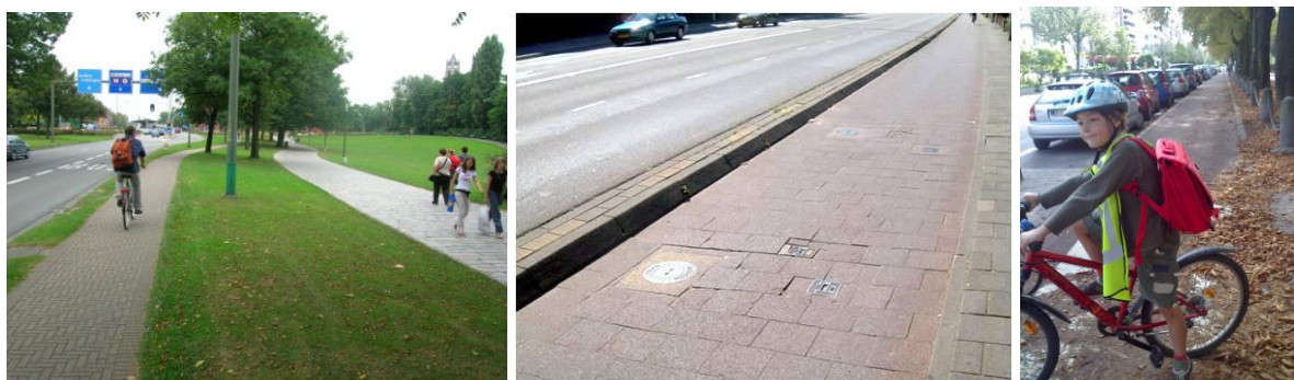
Cycle paths with verge partition, kerb partition and behind a parking lane (image source: T. Aspergers, P. Kroeze, D. Dufour)
