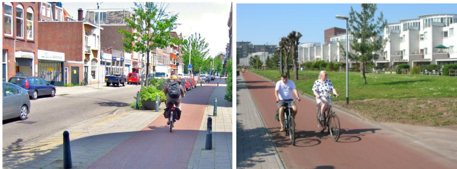
Well-segregated cycle tracks of different widths (image source: P. Kroeze, T. Asperges)
